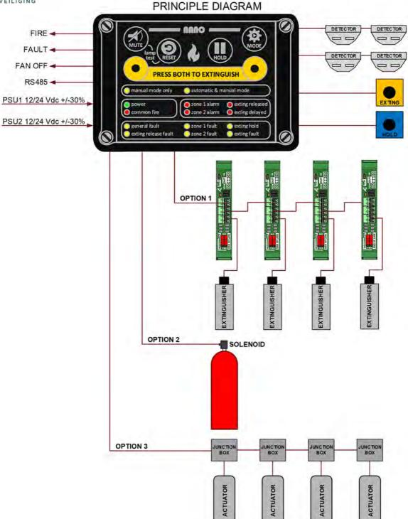
This schedule of working principles of the NANO fire extinguishing system is intended to be supportive of this leaflet and therefore not intended and suitable for technical realization. For more detailed information ask for the N2KB BV User Manual NANO-EN September 2022 V2.2
