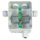
connection board is equipped with built-in security electronics, which ensures that all igniters of the extinguishing units are activated. Together with an end line switch, this option turns this system into a complete and reliable fire detection and extinguishing release system. The ETB extinguishers terminal board unit is available in a built-in 35 mm DIN rail version.
